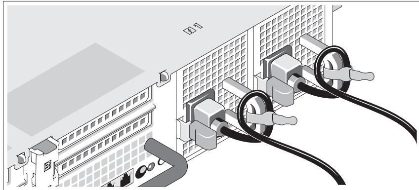
Bend the system power cable(s) into a loop as shown in the illustration and secure the cable(s) to the bracket using the provided strap.
